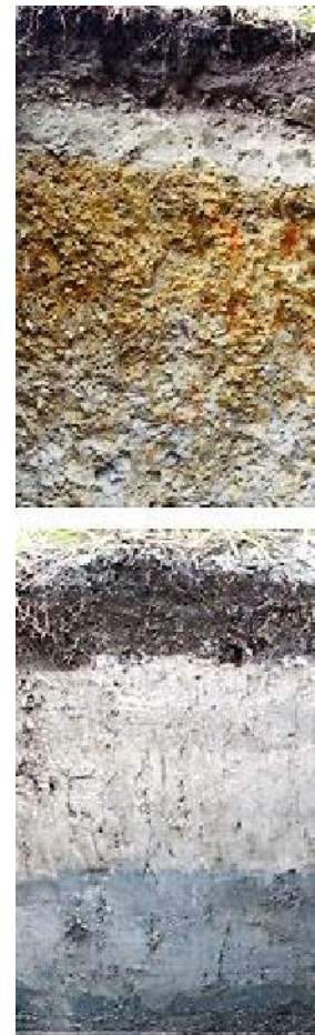
Figure 4: Images of redoximorphic features (top) and gleyed soil (bottom).
